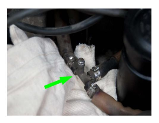
First, release (put a rag under) the fuel pressure with the little bleeder screw (green arrow)
