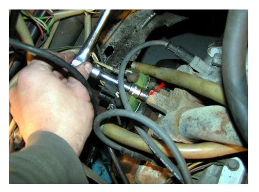
Remove the only screw that holds both injectors on the engine, slowly pull both injectors at the same time, being careful not to lose the 2 small sealing Orings (engine side) on the small end of the injectors. They may be stock on the engine, if so, remove them.
