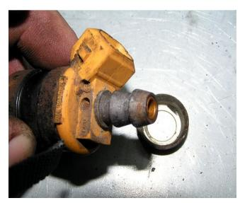
Cut 4 pieces of hose of the same length. Use an old one to measure length. Insert the new hoses into the injectors, affix a 5/16" FI clamp on each injector and secure those carefully.
