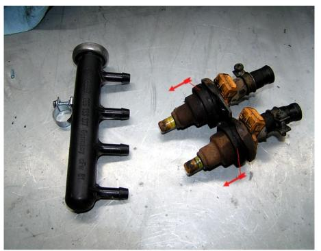
Remove the 2 big O-rings, the clamps and the metal holder.
