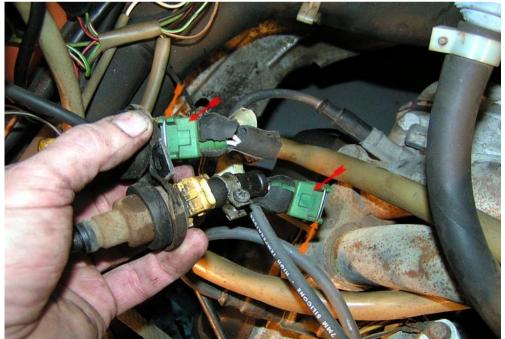
Unhook the 2 injector connectors by pulling the metal clip.
